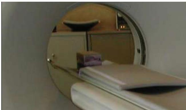
2. Place a metallic point marker at the center of the top of the stand. Use the couch movements to bring the metallic point marker to the isocenter of the CT scanner (figure 2). Conduct a test scan to confirm that the metallic point marker is at the isocenter. Adjust the couch required to bring the metallic point marker to the isocenter.
